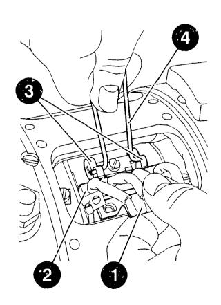
Detach all connections and unions at connecting ring (1) of excitation winding.
